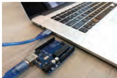
5-rasm. Dasturni Arduino UNO platasiga yozish.
